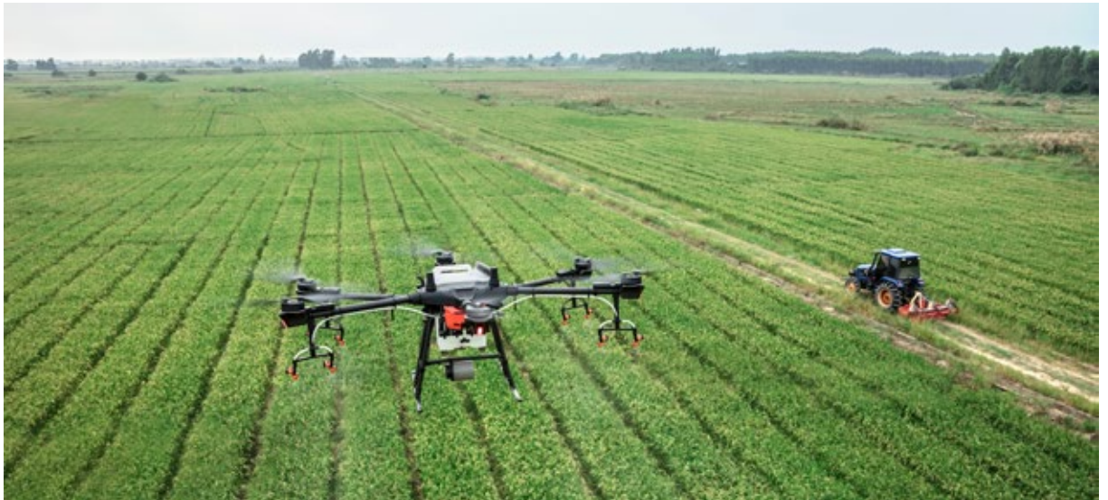
DJI Agras T16 drone used for precision spray application
